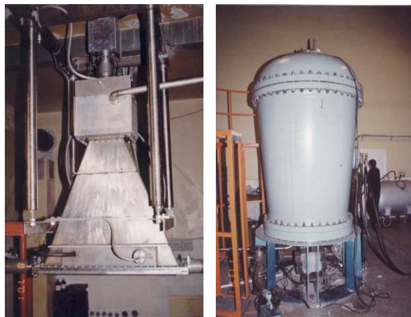
Figure 9: The 800~1200 KV 80 mA accelerator at LIMPR
