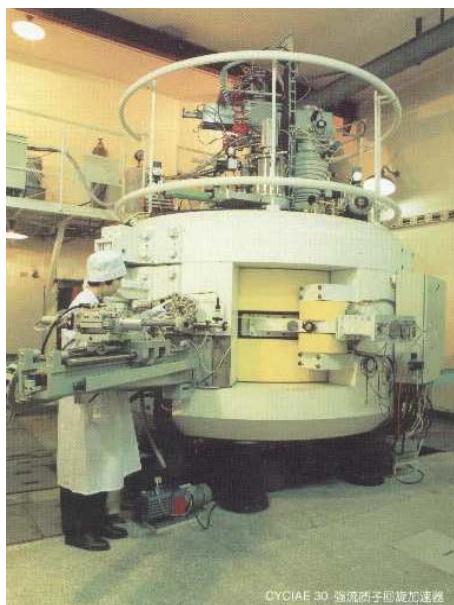
Figure 6: 30MeV Cyclotron (CYCIAE-30) made by CIAE.
