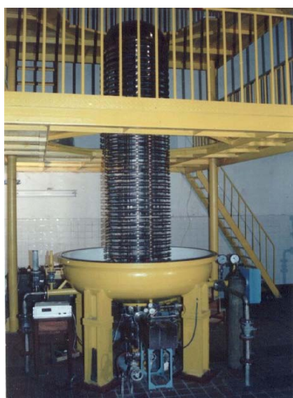
Figure 4: 3.0 MeV Dynamitron-type machine made by SINR.
