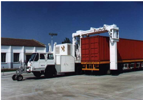
Figure 12: mobile container inspection system
