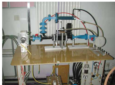
Figure 6: C-band 2.5MW RF test facility.
