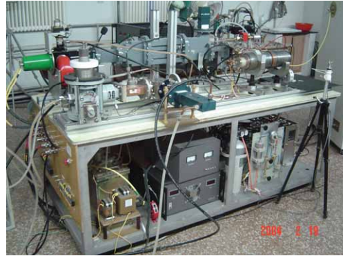
Figure 4: S-band 2.6MW RF test facility.
