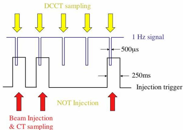
Figure 2: Timing of data acquisition.
