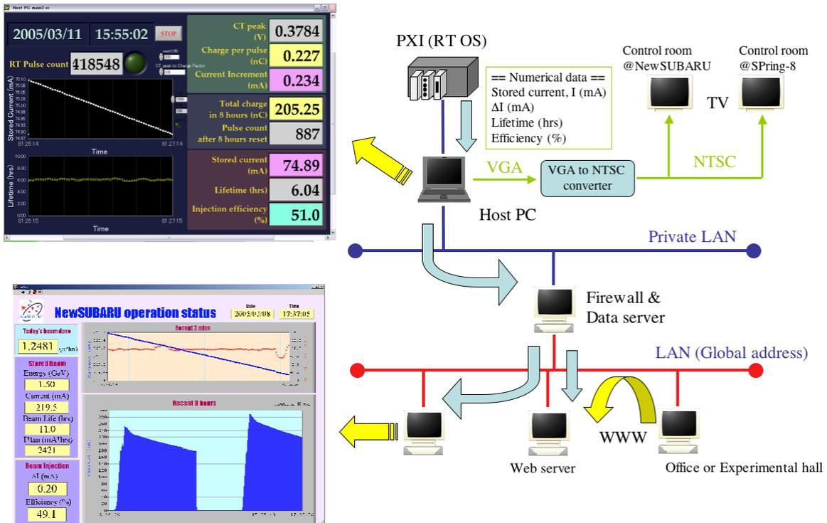
Figure 4: Network of PXI RT system and host PC.
