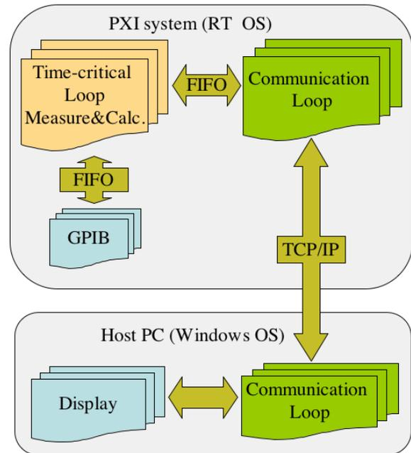
Figure 3: Software outline of RT system and host PC.
