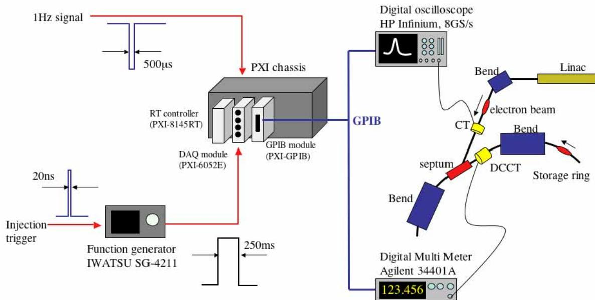
Figure 1: Hardware configuration of beam injection efficiency monitor.
