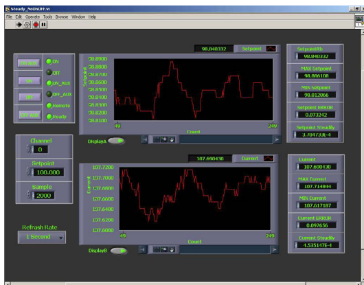
Figure 6: On-line test with a prototype power supply.
