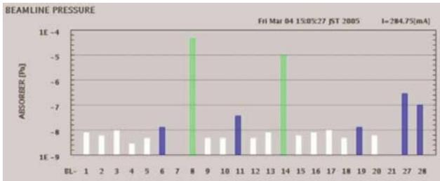
Figure 4: A screen shot of a console display for ultra-high vacuum of fifty beamlines.
