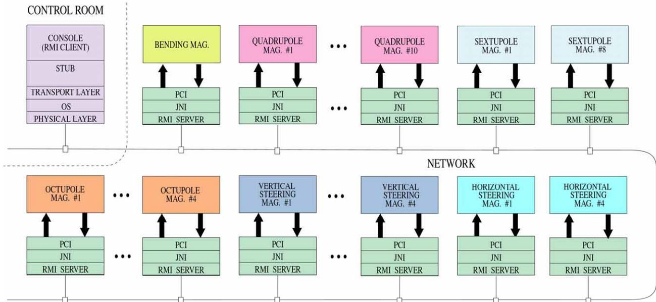
Figure 1: Remote Equipment using RMI for the 1.8GeV Synchrotron Radiation Source at TSRF.
