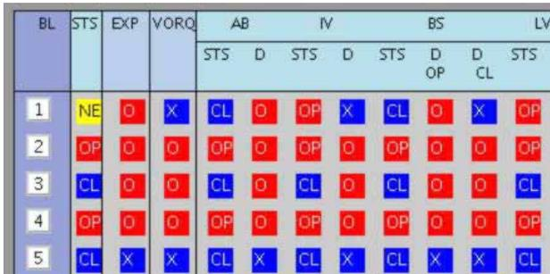
Figure 3: A screen shot of an operator console for emergency interlocks and summary status display for the beamline status.
