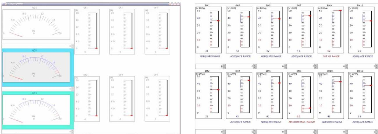
Figure 2: Screen shots of an operator console for a magnet controller.
