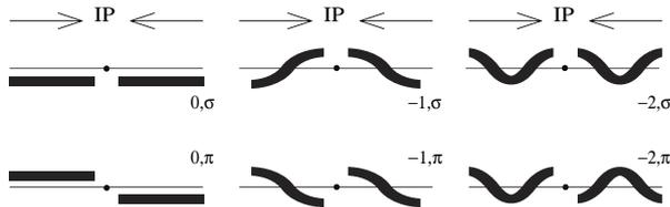
Figure 1: Naming convention for the synchro-betatron beam-beam modes.
