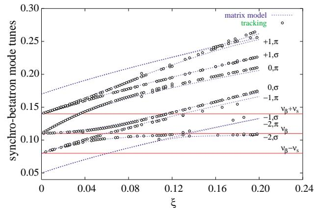
Figure 2: Synchro-betatron mode tunes vs. the beam-beam parameter  $\xi$ . Comparison of the circulant matrix model and tracking. Equal bunch intensities,  $\nu_\beta = 0.11$ ,  $\nu_s = 0.03$ , and the bunch length is  $0.7\beta^*$ .
