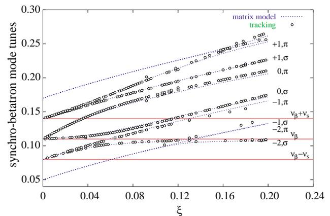
Figure 2: Synchro-betatron mode tunes vs. the beam-beam parameter  $\xi$ . Comparison of the circulant matrix model and tracking. Equal bunch intensities,  $\nu_\beta = 0.11$ ,  $\nu_s = 0.03$ , and the bunch length is  $0.7\beta^*$ .
