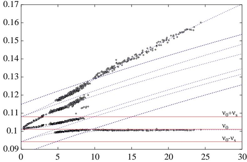
Figure 5: Measured (circles) and calculated (lines) synchro-betatron mode tunes vs beam current  $I$  (mA). VEPP-2M was operated with one  $e^+$  and one  $e^-$  bunches colliding at two IPs,  $\nu_\beta = 0.101$ ,  $\nu_s = 0.0069$ ,  $\beta^* = 6$  cm, and the bunch length was 3.5 cm.
