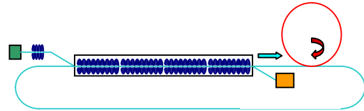
Figure 1. Schematic layout of the electron linac – proton ring collider.
