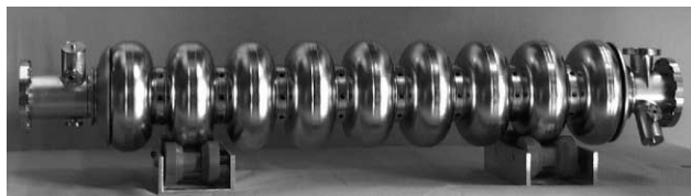
Figure 1: A TESLA niobium 9-cell cavity. The length of a cavity is about 1m.
