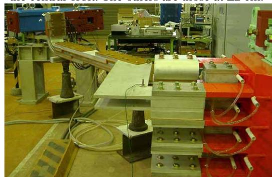
Figure 5: Completed dipole magnet connection to the pulse transformer with a bus-bar.
