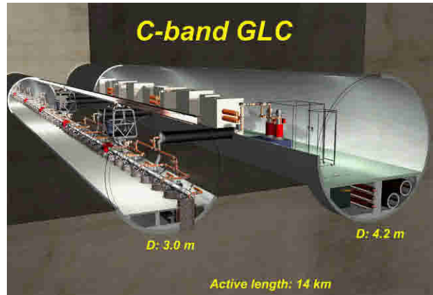
Figure 1: C-band main linac tunnels. The klystron gallery is 4.5-m in diameter and the linac tunnel is 3.0-m in diameter.
