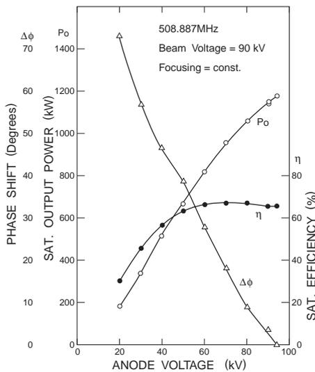
Figure 3: Performance as a function of anode voltage.
