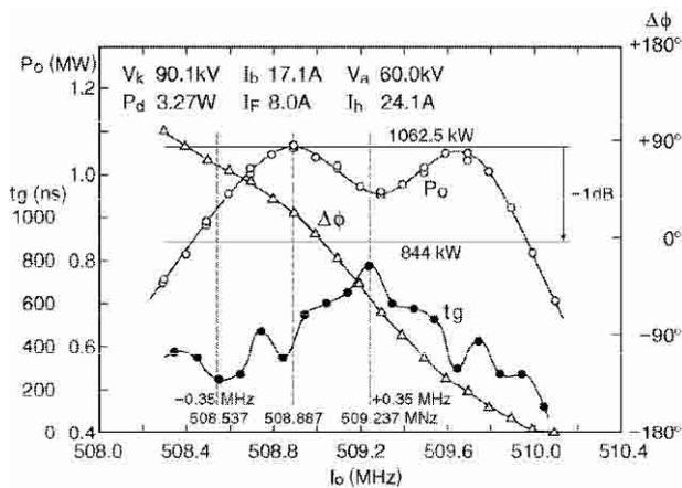
Figure 4: An example of instantaneous bandwidth characteristics of T41. The beam voltage,  $V_k$ , is 90.1 kV.
