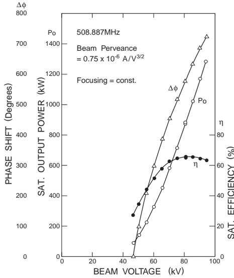
Figure 2: Performance of T41 as a function of beam voltage.
