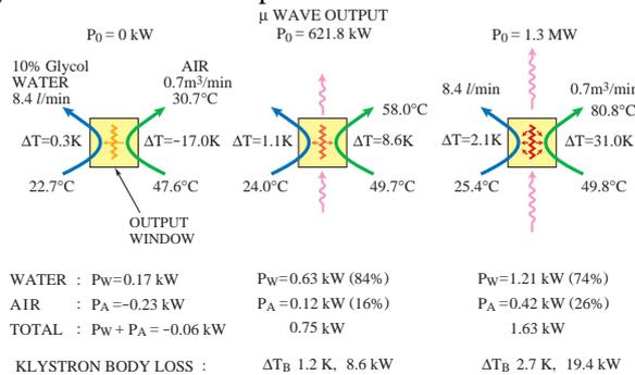
Figure 7: Hybrid cooling system of klystron output window.
