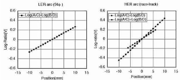
Figure 4: Log ratio value to the beam position on an axis of coordinates of LER BPM and HER BPM.
