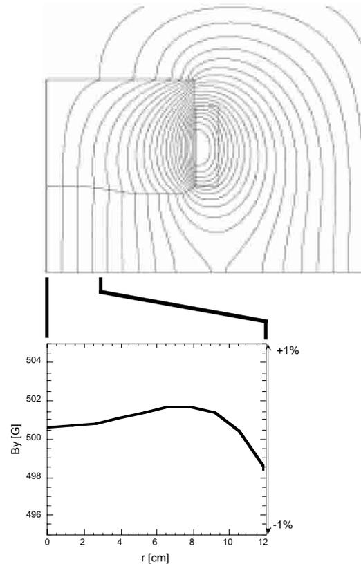
Figure 4 (a): Calculated field distribution in X-Y plane.
