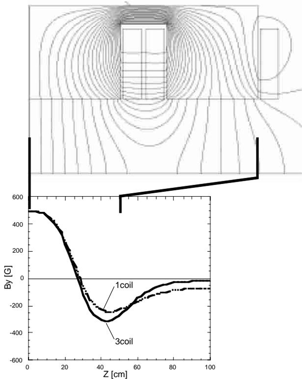
Figure 4 (b): Calculated field distribution along the beam line.
