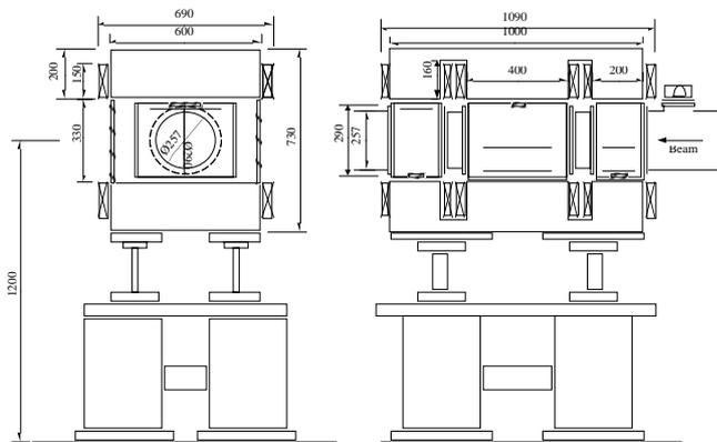
Figure 2: Schematic layout of the beam profile monitor. The proton beam ionises the residual gas atoms. The products are driven electrostatically towards the MCP detectors with gyromotion around the external magnetic field lines.
