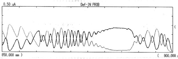
Fig.4 :  $^3\text{He}$  beam current as a function of a position of the beam probe of the AVF cyclotron
