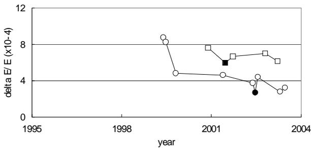
Fig.3: Observed energy spreads in each machine time for 400 MeV <sup>4</sup>He beam(circle) and for 210 MeV <sup>4</sup>He beam(square) . Filled symbols represent the best results.
