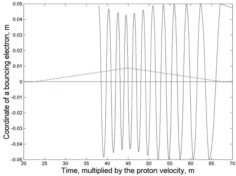
**Figure 1 Motion of an electron in the fields of the proton beam.**
