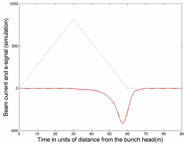
**Figure 2 Proton bunch longitudinal distribution (blue) and the electron signal (red).**
