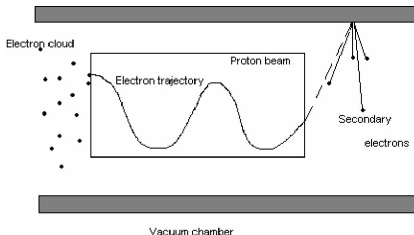
**Figure 4 Schematic motion of electrons in the field of the proton bunch.**
