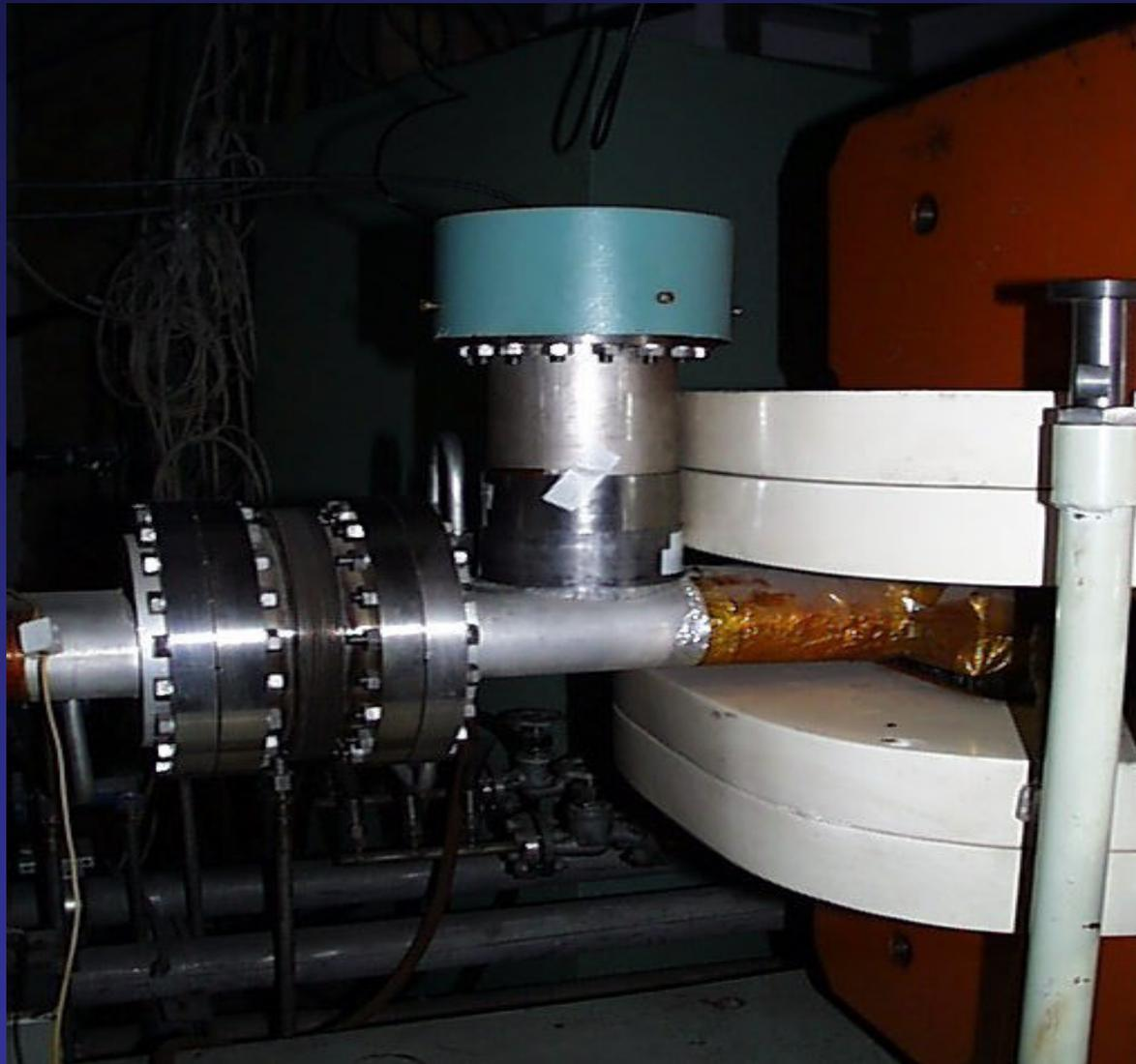
The shielded PE detector after mounted on the BEPC storage ring<sub>5</sub>
