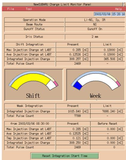
Figure 5: NewSUBARU injection charge limit panel.
