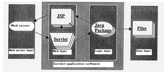
Figure 3: The class architecture of servlet applications
