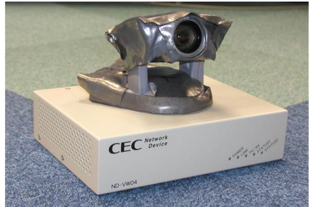
Figure 1: The CCD camera "Canon VC-C4" with lead covers. And the network camera server "CEC ND-VW04"
