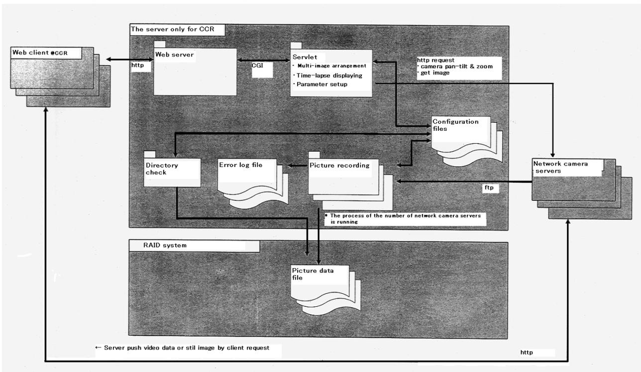
Figure 2: The flow of process
